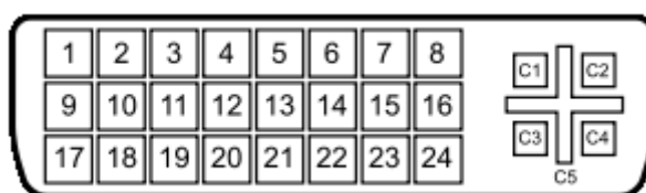
< Figure 3 > DVI 29Pin I Type Female Connector
